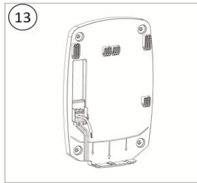
13 Route the wires through the Plug-in base as shown on the picture
