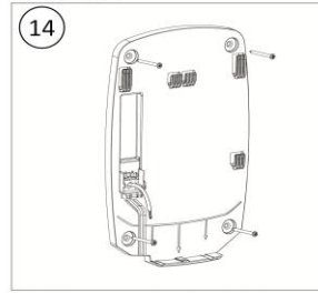
14 Screw the Plug-in base to the wall(x4)
